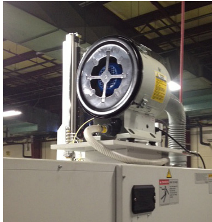
This image shows a single unit source capture mist collector with the mist intake hose connected to the machine enclosure.
